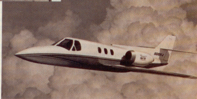
In 1968, Cessna launched the first civilian jet, the FanJet 500 (right). Its 2,200-pound thrust JT15D-1 twin-spool front fan engines were lauded for their efficiency (above).
